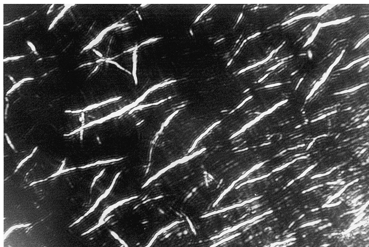
Fig. 3. Bâtonnet texture of PEI 5b observed upon slow cooling from the isotropic melt.
