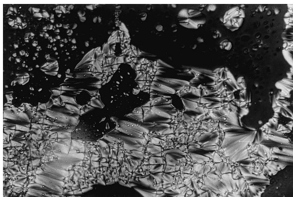
Fig. 4. Fan-shaped texture of PEI 5b obtained upon further cooling of the bâtonnet texture (Fig. 3).
